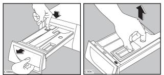
To aid cleaning, the top part of the additive compartment should be removed.
